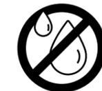
A water drop in a barred circle symbol is to warn the user of a potential risk of water damage to the product, and electrical shock
